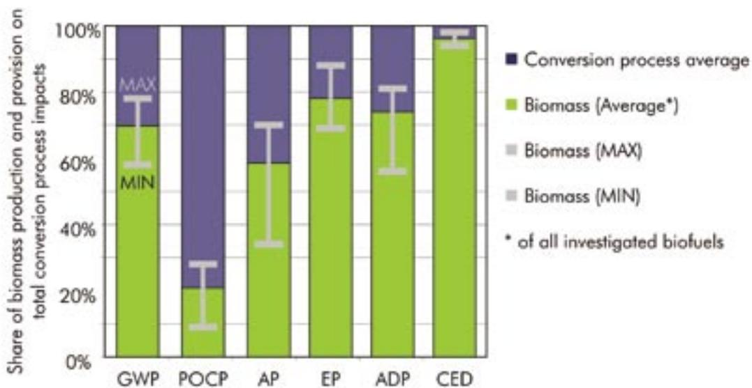
**Figure 4:** Share of biomass (production and provision) in total conversion processes (incl. fuel distribution) impacts. GWP: Global Warming Potential; POCP: Photochemical Ozone Creation Potential; AP: Acidification Potential; EP: Eutrophication Potential; ADP: Abiotic Resource Depletion Potential; CED: Cumulative Energy Demand
