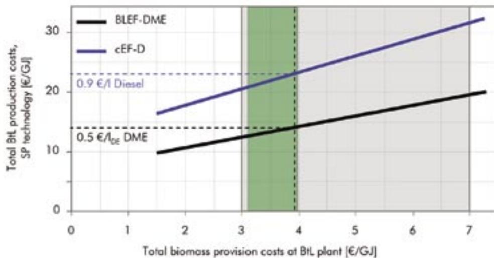
**Figure 8:** Influence of the cost of biomass on the BtL production costs of the examined BtL concepts BLEF-DME and cEF-D. The dashed line is the 2007 price for wood chips in Sweden (3.9 €/GJ or 72 €/t<sub>DM</sub>), the grey shading illustrates the bandwidth of estimated cost for forest residues in SP (2004), the green shading is the bandwidth of estimated energy crop cost in S1 (2020). 1 €/l<sub>Diesel Equivalent</sub> is approximately 28 €/GJ
