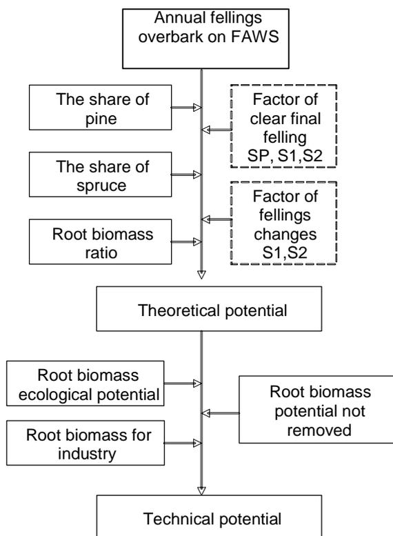
Figure 2. Scheme of root biomass assessment
